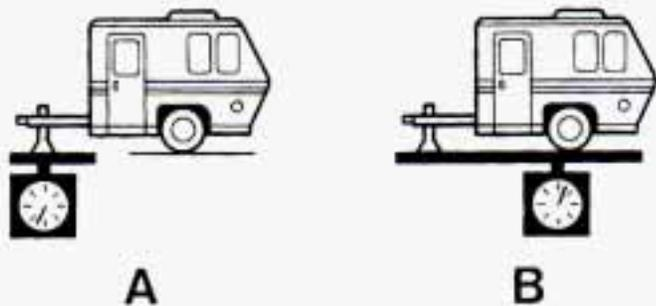
If you’re using a weight-carrying hitch, the trailer tongue (A) should weigh 10 percent of the total loaded trailer weight (B). If you have a weight-distributing hitch, the trailer tongue (A) should weigh 12 percent of the total loaded trailer weight (B).
