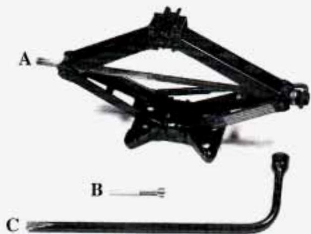
The tools you'll be using include the jack (A), extension and protection guide (B) and wheel wrench (C).
