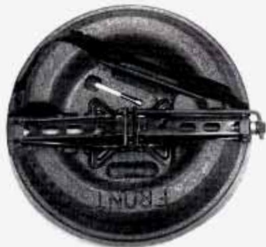
3. Turn the nut holding the jack to the left and remove it. Then remove the jack and wrench.
