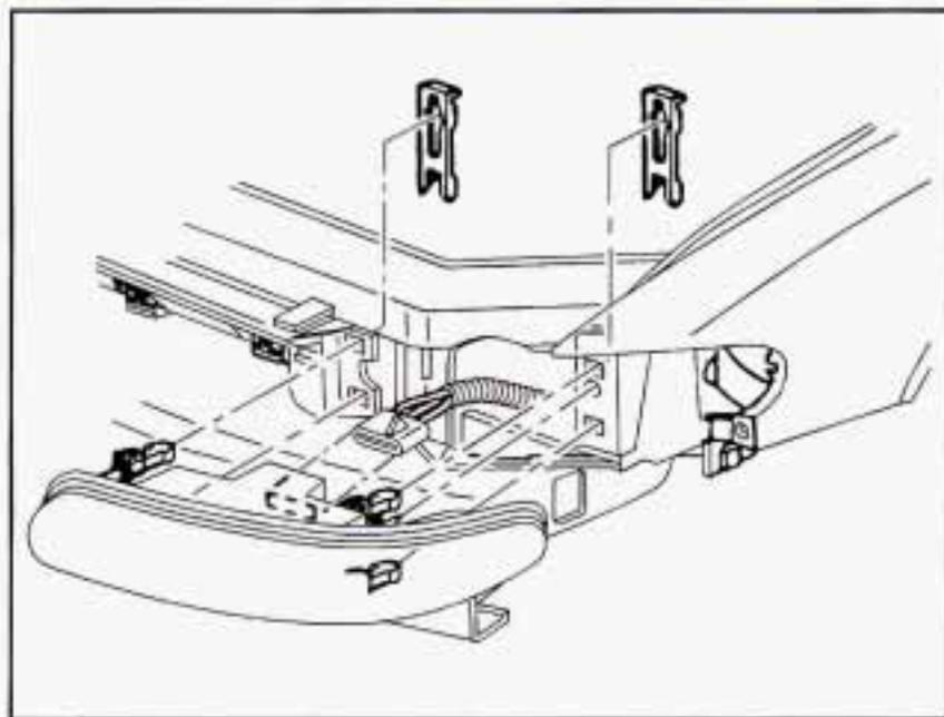
1. Pull up on the headlamp retainers to release the assembly locator tabs.
