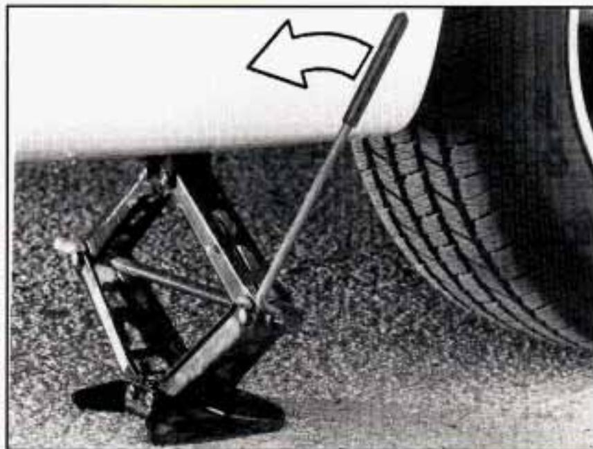
9. Lower the vehicle by turning the jack handle to the left. Lower the jack completely.
