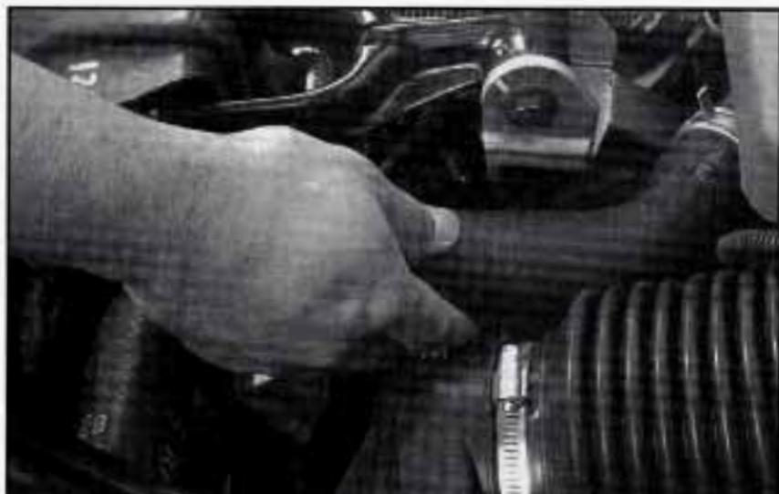
6. Then fill the coolant recovery tank to the COLD mark on the overflow hose in the coolant bottle.
