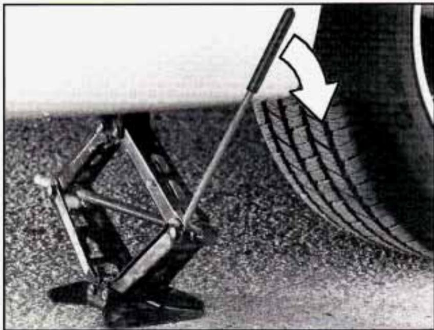
5. Raise the vehicle by turning the jack handle to the right. Raise the vehicle far enough off the ground for the spare tire to fit under the vehicle.
