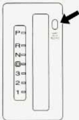
If your vehicle's battery should go dead or there is a lack of electrical power, there is an access slot that will allow you to override the PARK (P) lock if your shifter is stuck in PARK (P).
