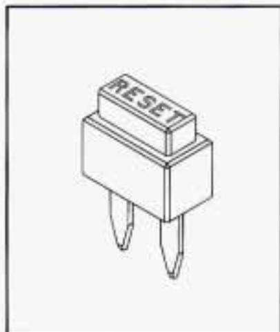
The red RESET button is located inside your instrument panel fuse block. (It's the first button in the top row of the fuse block.)
